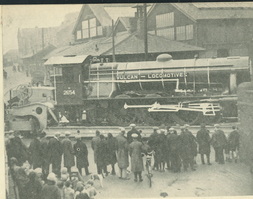
STANDARD 4-6-2 INDIAN PASSENGER LOCOMOTIVE ON ROAD LORRY EN ROUTE FROM NEWTON-LE-WILLOWS TO LIVERPOOL.
